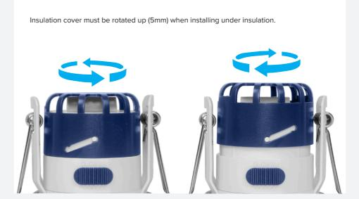
The Inceptor Milli's rotatable insulation cover introduces a practical solution for installation challenges, offering an extra 5mm clearance when placed under insulation. By accommodating insulation materials more effectively, the Inceptor Milli ensures optimal performance. Unrestricted airflow around the fixture helps manage heat dissipation, contributing to the longevity and efficiency of the downlight.
