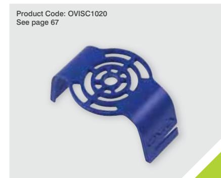
Sold Separately - the removable Insulation Support Bracket has been developed to allow installers to lay thermal insulation directly over the top of the Inceptor® Nano<sup>v2</sup>. Creating a 20mm air-space above the driver allows air to circulate and cool, therefore the driver dissipates heat more effectively and in-turn lets the luminaire run cooler.
